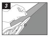
Note\* To secure edges cut (2) SLF 12" strips. Cut the SLF coil strips on both SLF strips to equal 4 coil strips to secure edges.
