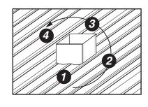
Stretchable Linear Flash (SLF) installation has 4 steps starting from the bottom of application (lower side of the roof slope) going counter clock wise.
